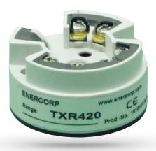
The TXR420 is a digital temperature transmitter and can be PC programmed to be used with a Pt100 RTD at various temperature ranges. This device is protected against reverse polarity and has sensor fault detection built in.
