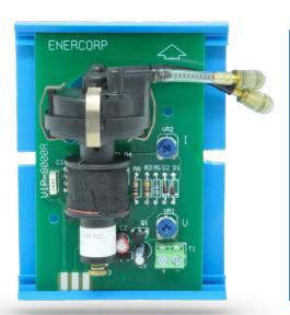
The VIP-9000 is an I/P or V/P transducer for interfacing electronic control panels to pneumatic valves. A 4...20mA or 2...10VDC input signal is converted into a 3...15psi pneumatic signal to position dampers and valve actuators.
