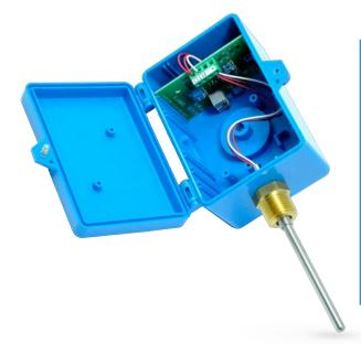
The pipe immersion temperature sensor is used to measure the temperature of fluids or gases in pipes. The spring loaded probe provides good thermal contact with the mating thermowell allowing for fast and accurate measurements.
