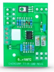
The TT-R-100 is used to convert a 2 wire Pt100 RTD temperature sensor to a 4...20mA signal. The output is proportional over a selected span and a diode protects against reverse polarity.
