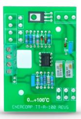
The TT-R-100 is used to convert a 2 wire Pt100 RTD temperature sensor to a 4...20mA signal. The output is proportional over a selected span and a diode protects against reverse polarity.
