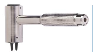
This hammer electrode with hatchet-type edges is designed to be used for softwood and surface contact applications, and must be driven into the wood across the grain. The electrode is driven into the wood by the user with a hammering motion.
