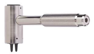
This hammer electrode with hatchet-type edges is designed to be used for soft and hard wood. The solid hammer head is to be placed against the wood and driven into the material with blows from a hammer over the entire length of the wood.
