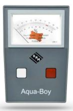
The LM series are highly accurate and portable moisture meters specifically designed for leather manufacturing. With instantaneous analogue readings, a centesimal scale and compatible electrodes, these devices have numerous applications for the textile industry.
