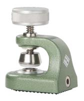
This electrode with a friction clutch allows adjustment of a constant pressure. For measuring materials in sheet form such as: cardboard, paper, leather, textiles or veneers.
